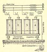
Fig. 178.—Schematic diagram for an ungrounded neutral three-phase electrolytic protector.
